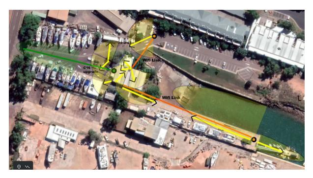
Attachment B: CCTV Plan – Positioning and Reach of Internal Cameras
